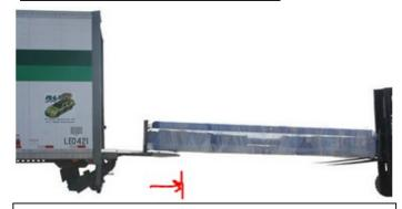
3. If there's room, pull the skid off the truck to where the end of the skid is resting on the liftgate. Otherwise, the driver can drive the truck slowly forward until the end of the skid is on the liftgate.
